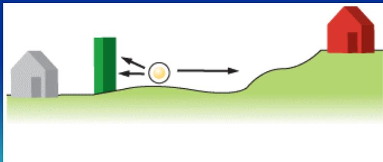
It is common to see parallel sound walls on roadways. Reflective parallel sound walls potentially reduce the walls acoustical performance. The net result is less than optimal performance and increased noise levels on and adjacent to the roadway.
