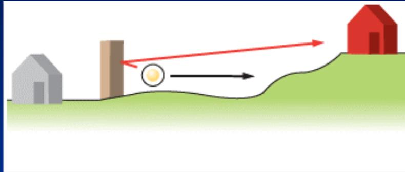
Using an absorptive sound wall shields the house at the same grade as the roadway and does not reflect noise up towards the house on the hill. Both houses are protected from the roadway noise.
