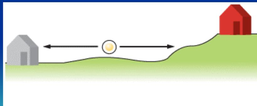
The addition of a reflective sound wall shields the house at the same grade as the roadway. Unfortunately, the reflections from the wall directly impact the house on the hill that was previously not impacted by the roadway noise. This situation depicted usually increases the noise level by 3-5 dBA for the house
