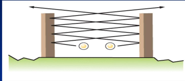
Absorptive parallel sound walls reduce reflections and are able to maintain the effectiveness of the barrier. In addition, the noise level on the freeway is reduced.
